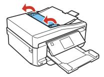
9. Carefully remove any jammed paper from beneath the ADF.
